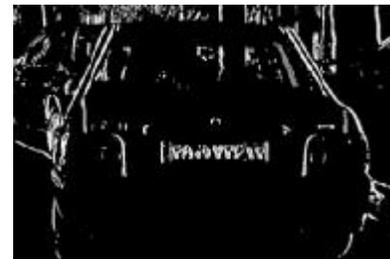
*Figure 3.* Vertical edge detection result
