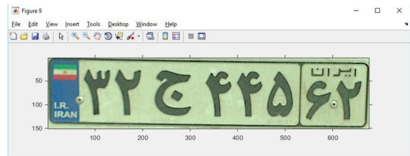
Figure 14. Extract plate using morphology method
