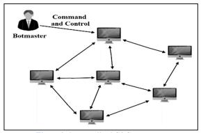
Figure 2: Decentralized C&C structure
